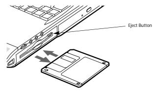
Figure 4-2 Loading/Ejecting a 3.5" Floppy Disk
